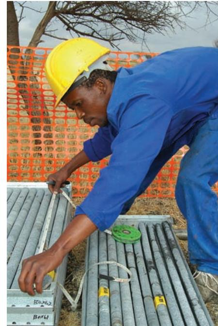
Samples of rock from the exploratory drilling being measured before going for analysis
