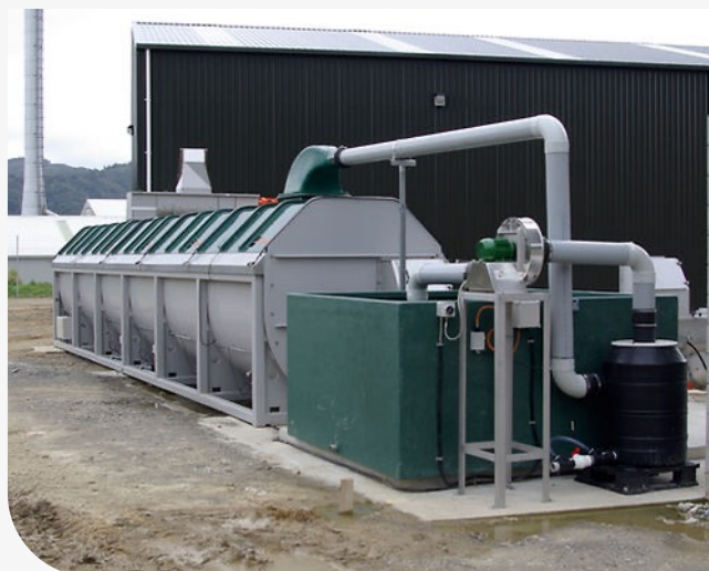
In-vessel composting. Source: Global Composting Solutions .
