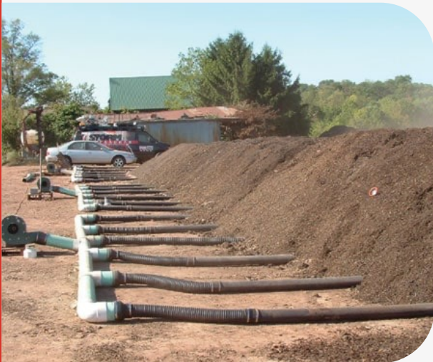
Static pile composting. Source: Waste Advantage .
