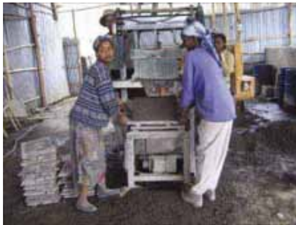
Hollow concrete block production by a small enterprise for housing development in Addis Ababa, Ethiopia.
